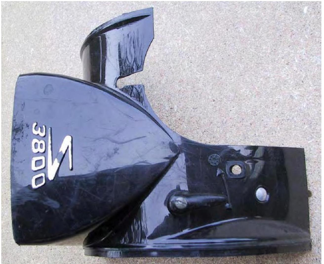
The carburettor guard is now sourced from the 5000. It has two mounting holes – one 6mm and one 8mm.
