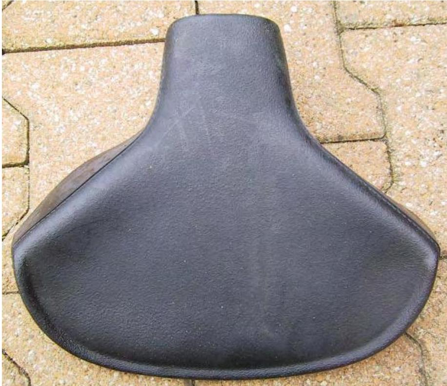
**The older seat cover branded “Brown” with a line-type grain surface continues to be fitted as standard.**
