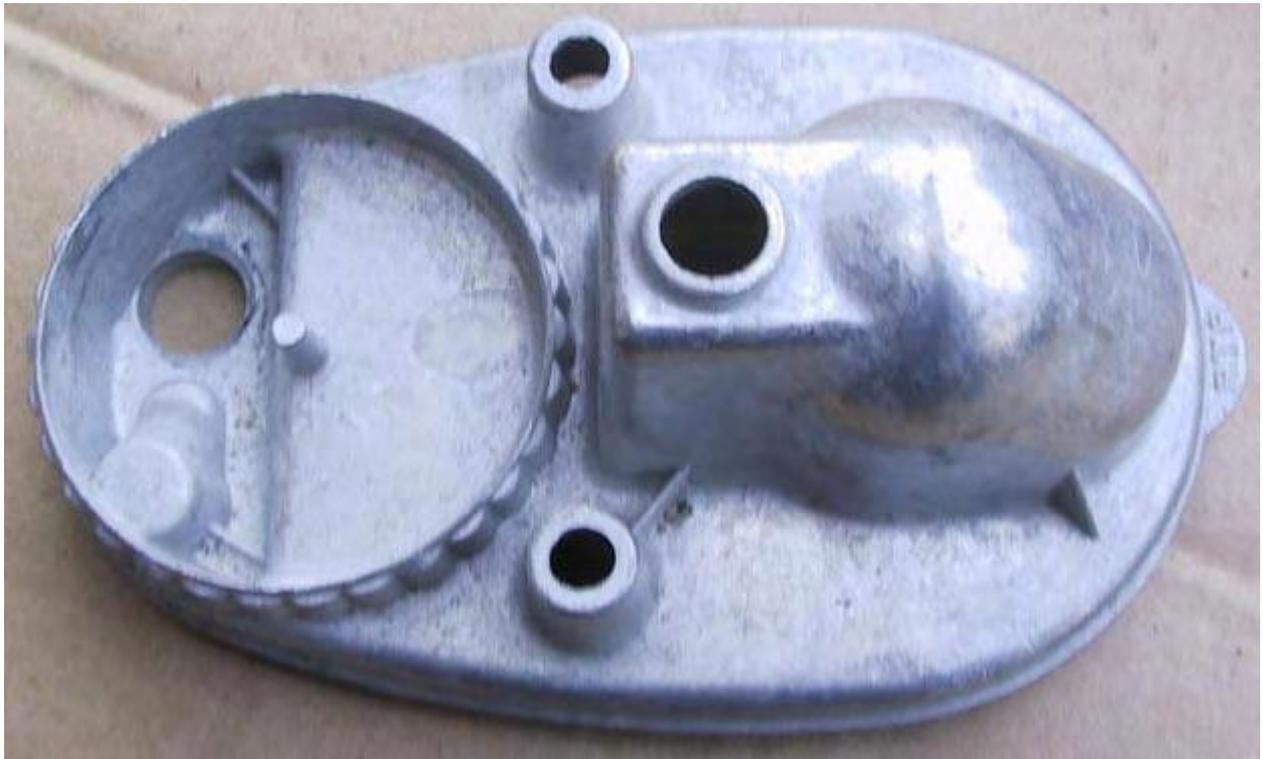
**The tank lid gets a ventilation hole on both the 5000 and 3800.**
