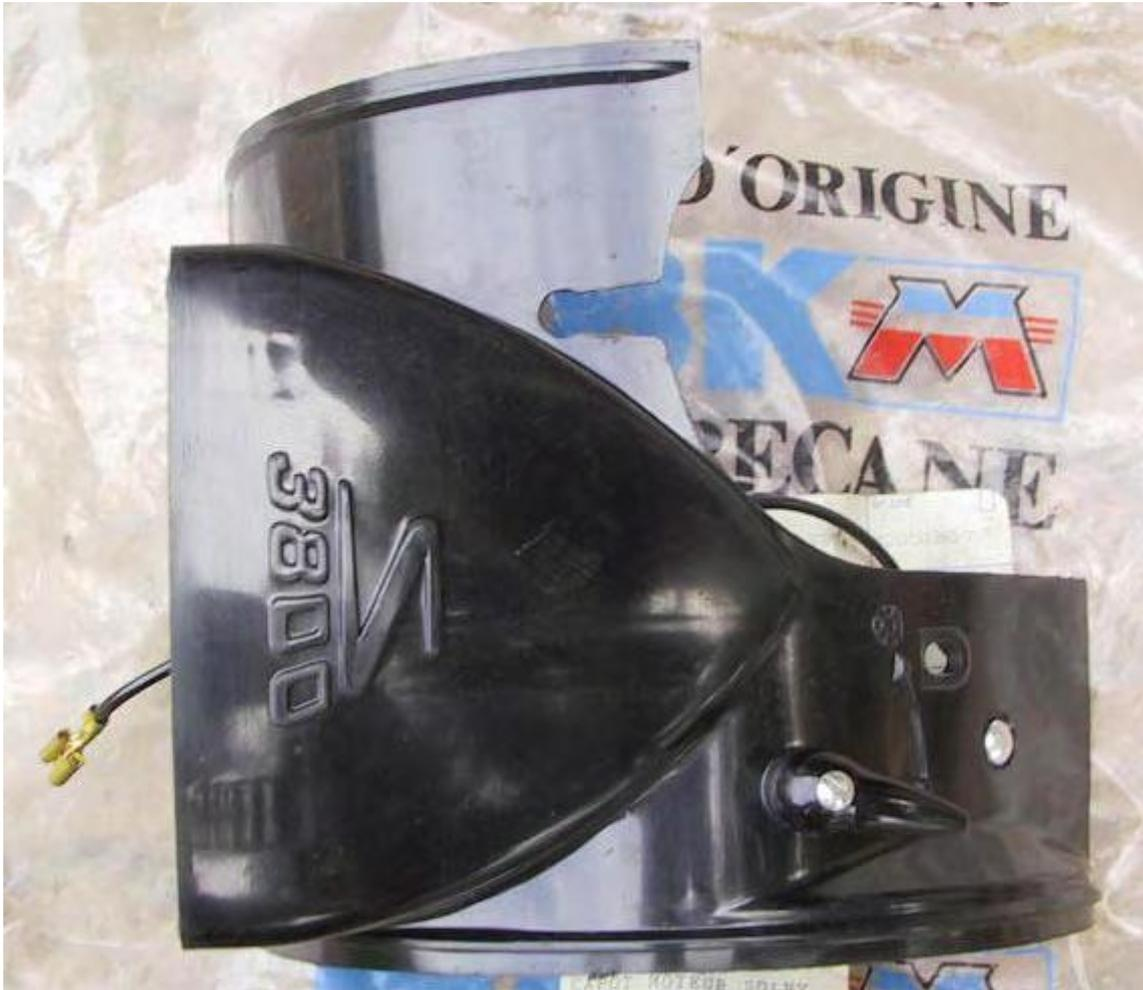
Internal ribs stiffen the light mounting to compensate for the additional weight of the glass lens.
