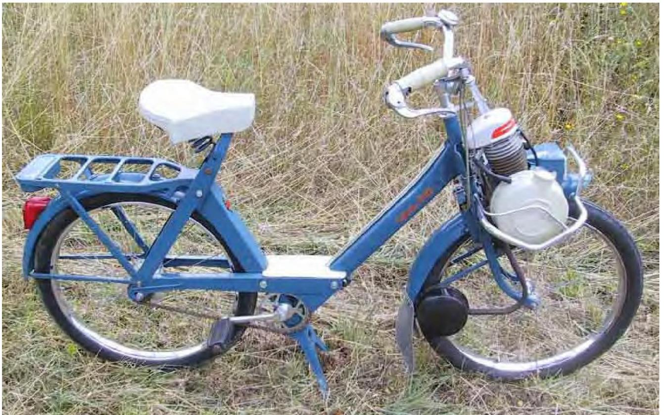
**Seat cover, handle grips, footplate, flywheel cover and tank are made from light grey plastic.**
