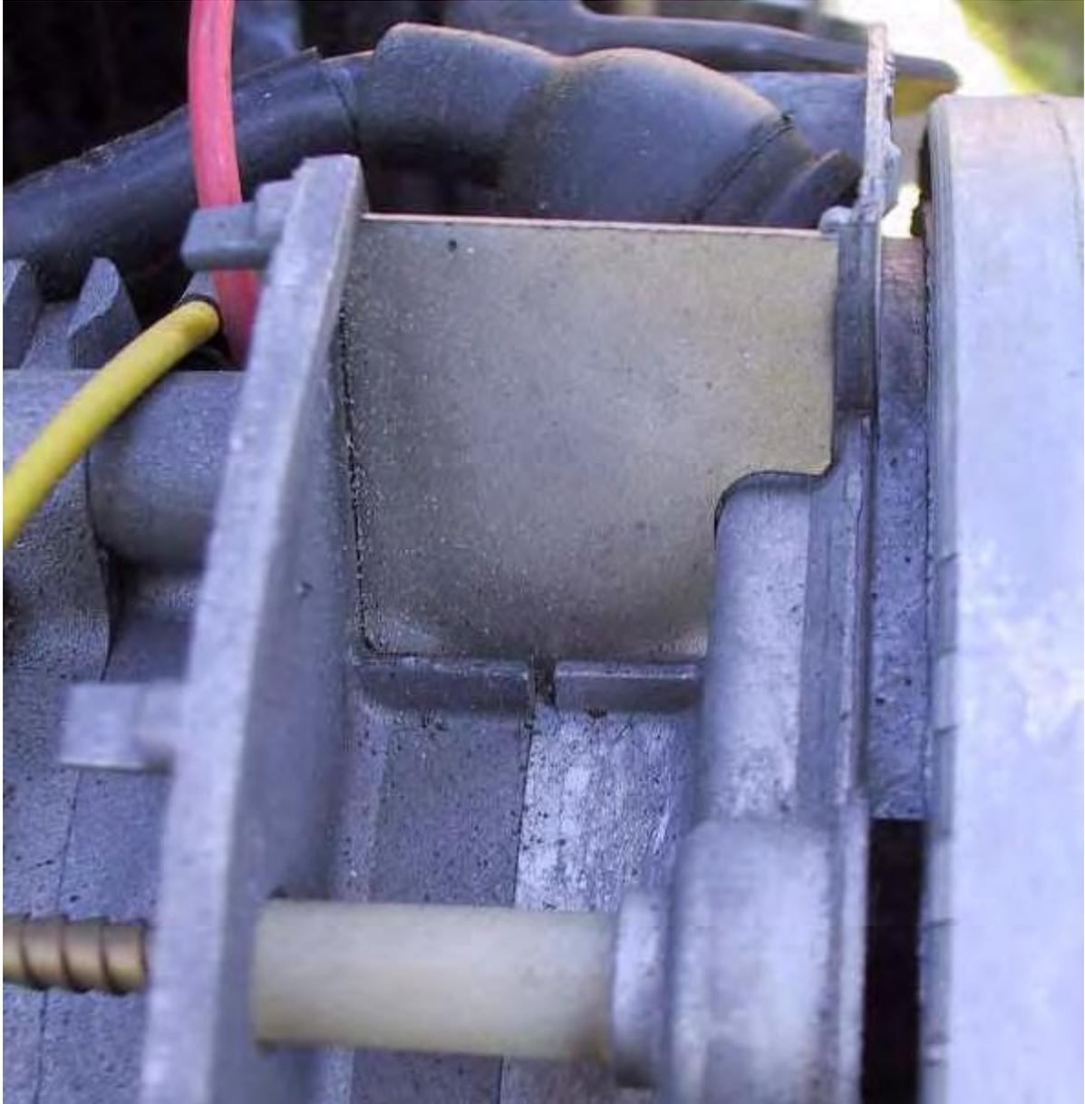
The stator is modified: there are now to small ribs near the bottom and one under the condenser.
