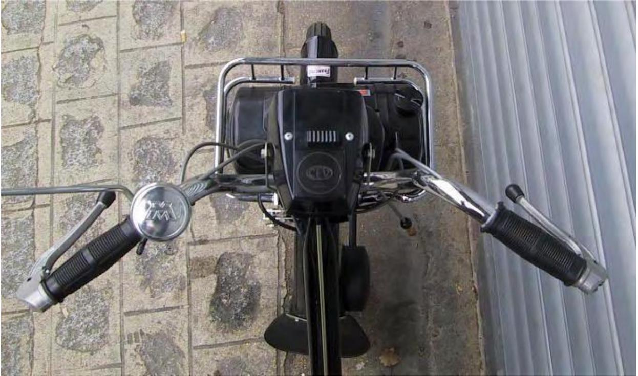
**The brake levers get black rubber balls fitted to their ends.**
