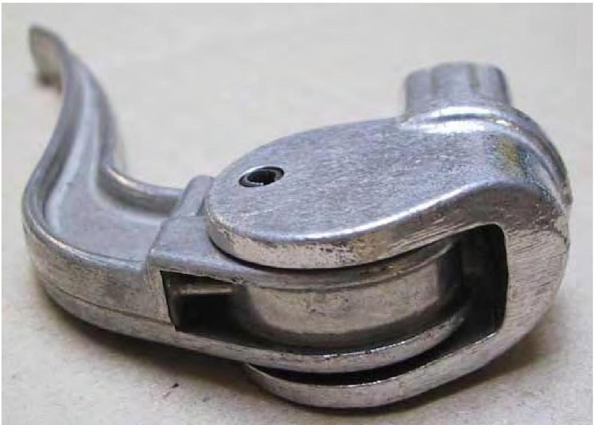
The engine cover is now fixed with a special bolt that also removes the dirt from the friction roller space, in order to make the light switch more reliable.
