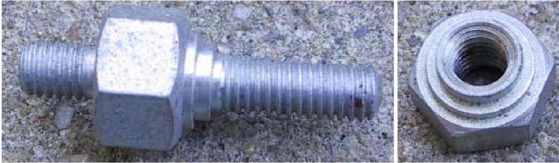
**The 14mm AF Bolts on the forks are also replaced with 13mm AF ones from the 5000.**
