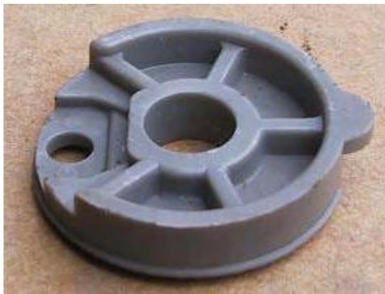
The headstem bearing nut loses its serrations, the wavy spring washer disappears and the octagonal nut is now taller. These new parts are fitted at the Tours factory from November 1966 and are generally fitted from April 1968.
