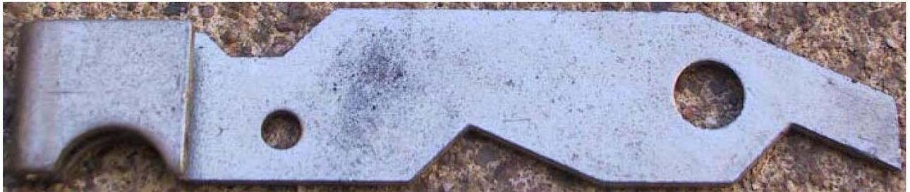
Another change of the motor cover: A flat cable connector 5mm wide for the taillight connection is fitted to the light switch blade instead of on the globe socket as was the version by Cibié.
