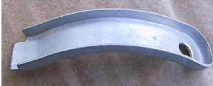
**New luggage carrier: the two mounting holes for the rear stays have been moved forward by 8 mm.**
