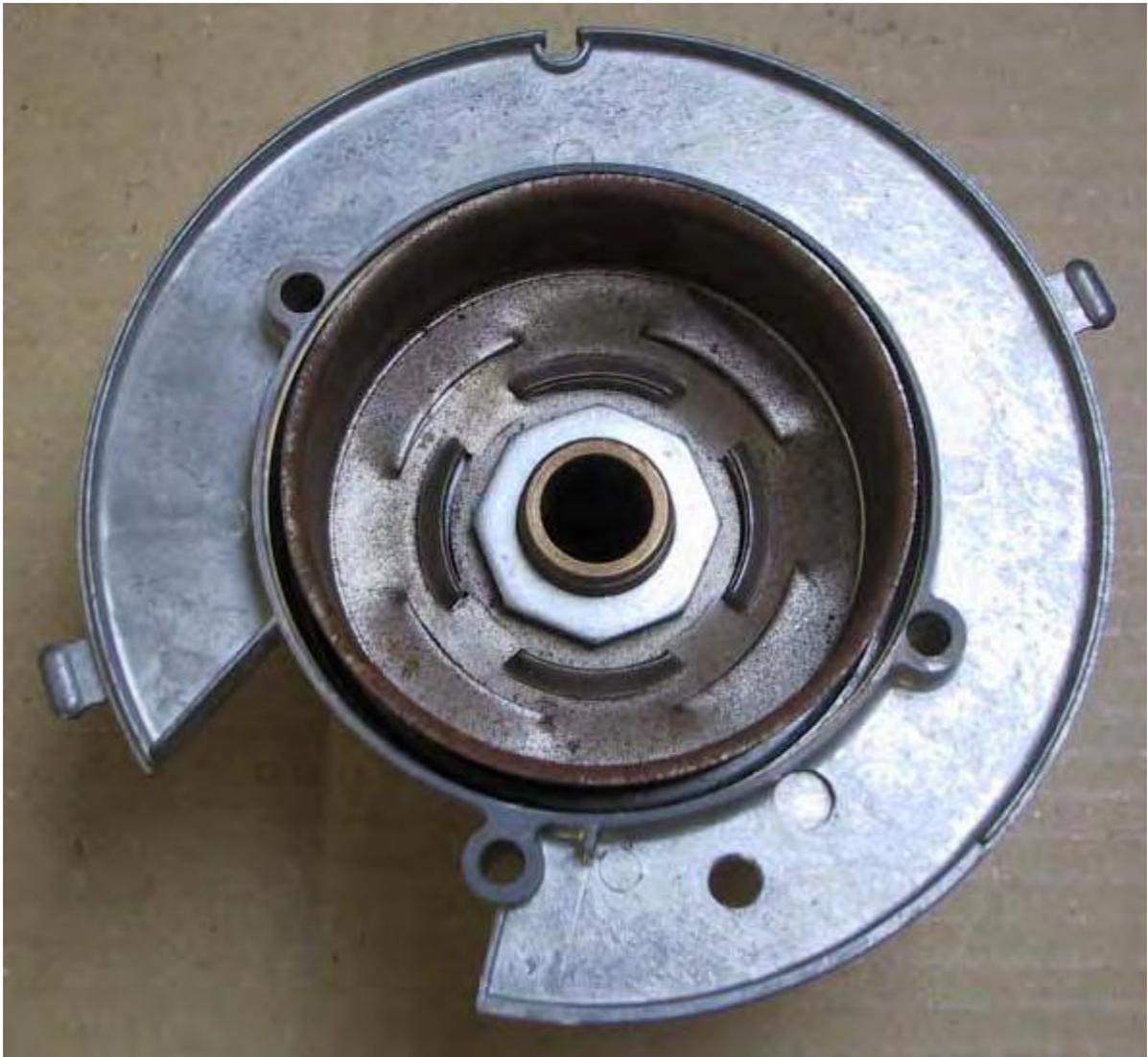
The clutch drum is secured to the friction roller with an octagonal nut of 37 mm
