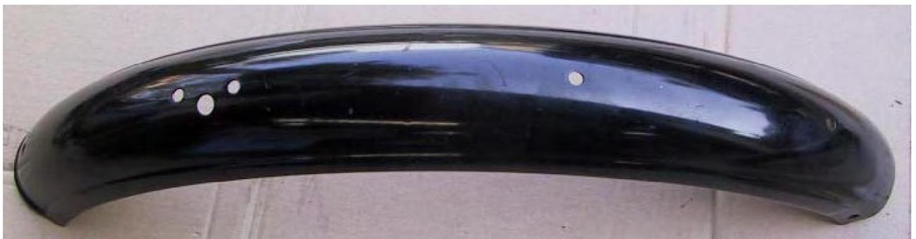
**New paint produces a higher gloss. It is sprayed over a white base coat.**
