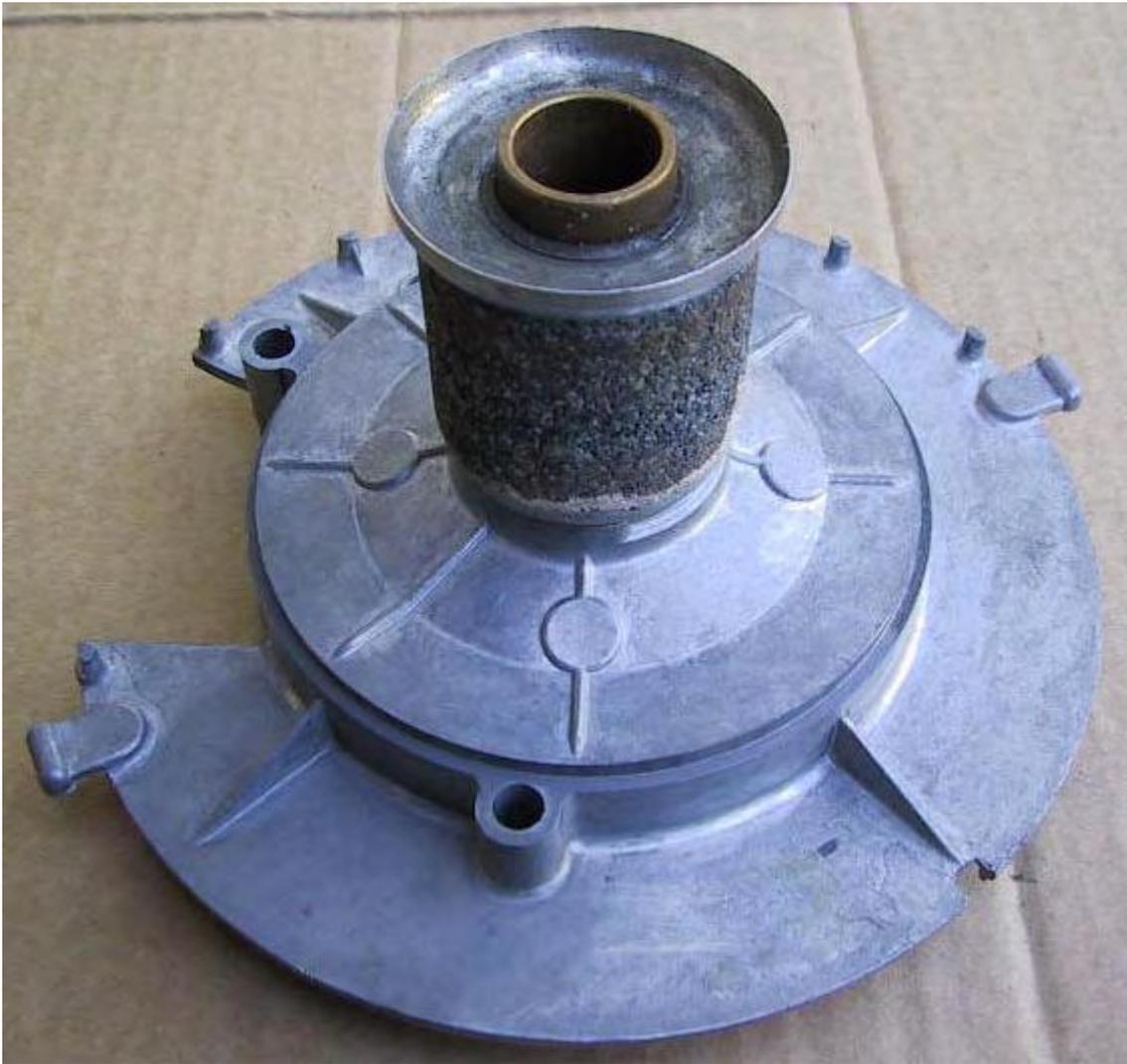
**A new muffler is fitted.**
