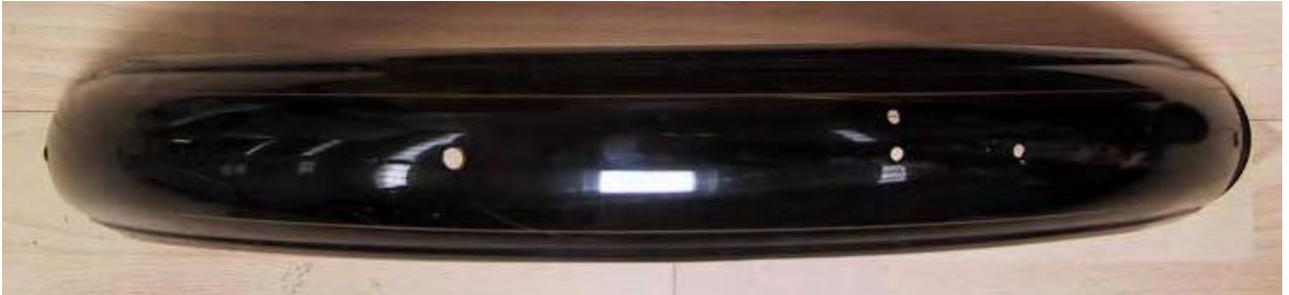
**The front mudguard is extended and forms a protective shield between the exhaust gases and the mud flap.**
