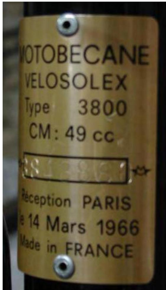
The engine numbers are now stamped onto a small aluminium label with is riveted to the crank case.
