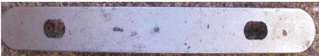
**New read mudguard stays. The bent ends are several mm longer.**
