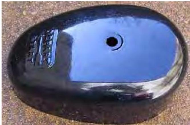
**The crank case now has a slot which is used to secure a spring hook-end on the Micron.**
