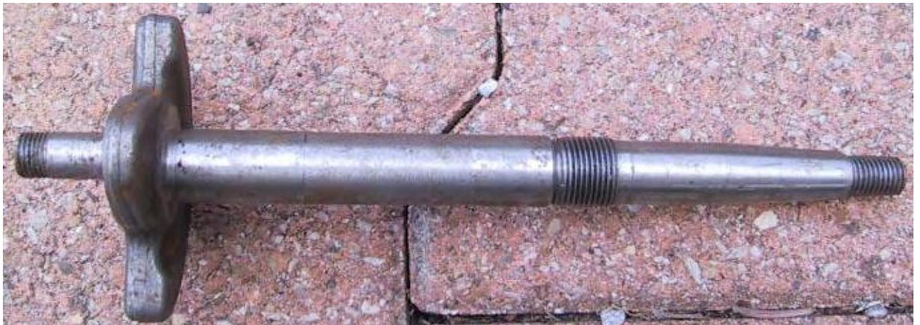
The friction roller runs on 2 bronze bushes and has a smaller diameter:
