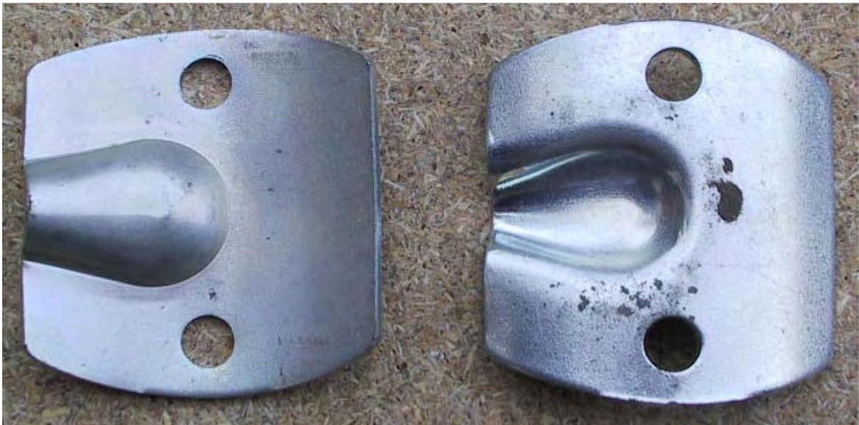
**The rear mudguard is altered to suit the new mounting holes required.**
