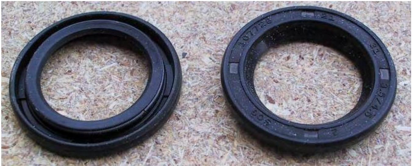
**New smaller seal: 31mm OD in place of the older 40mm OD one.**
